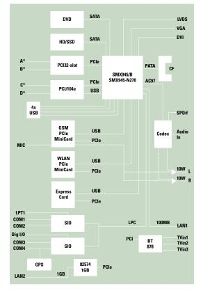
\*A, B, C, D interfaces depend on the built-in PCI/104e cards or their respective slots
