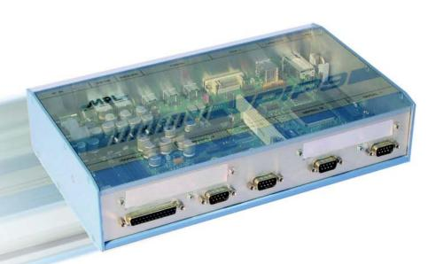
PIP9 dimensions: 270 x 162 x 62 mm (L x W x H) Weight: 2,2 kg, rugged aluminum housing with best EMI/RFI protection (internally chromated, externally powder coated or eloxated)
