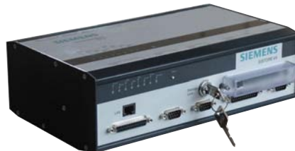
OEM-PIP with lockable PC-Card slot
