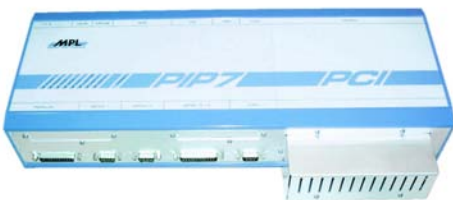
PIP7 with 2 standard PCI slots inside
