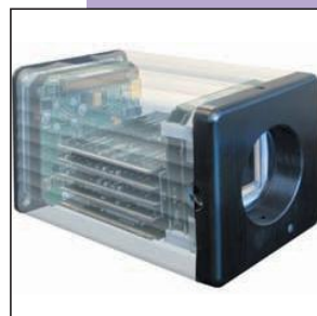
Vision: High Speed Camera up to 32'000 pictures/second, 100G shock
