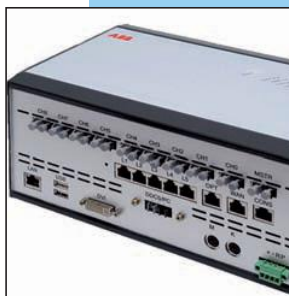
Pentium M 1.8 GHz with integrated fibre optic distribution, firewall
