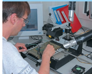
BGA re-work station
