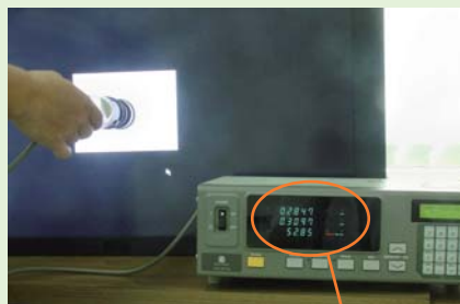
1000 nits brightness (Measured by 20:1 attenuator)
