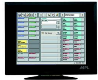
PIP8 with 12" XGA display and touch, IP65 all around, fanless, noiseless
